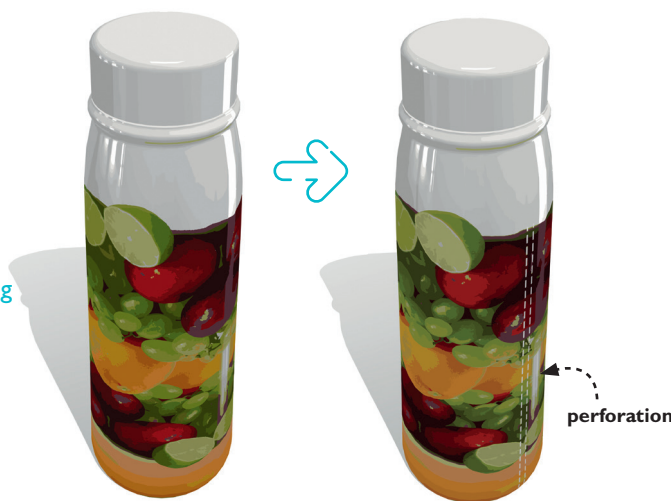
Vial body in PET + sleeve in OPP
